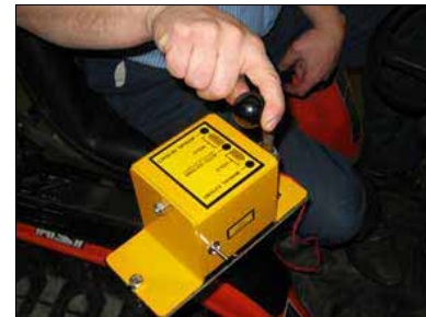
Pull R/E Control Lever back to move out of the row. (retract)
