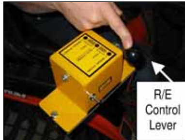
Push R/E Control Lever forward to move into the row. (extend)
